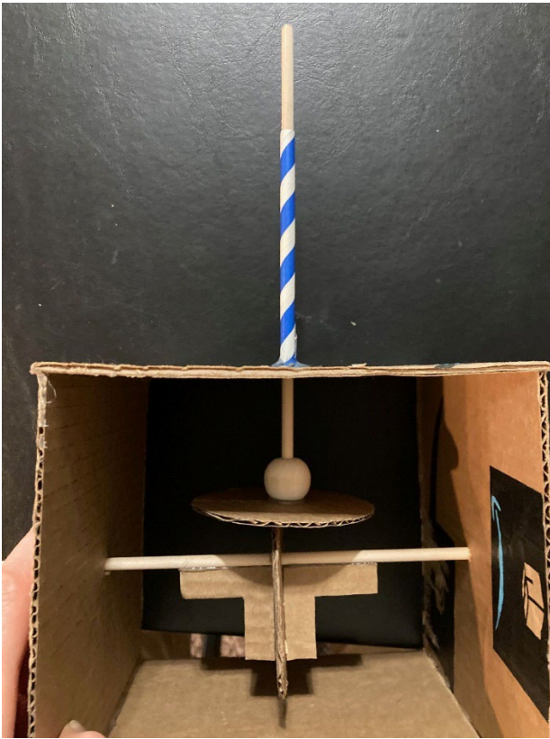
Example of completed cam and rotating axle system for the cardboard bird automaton.
